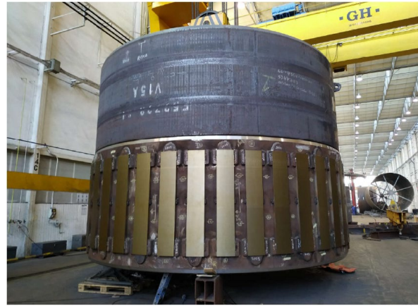
Kiln tyre shell section with supporting blocks
