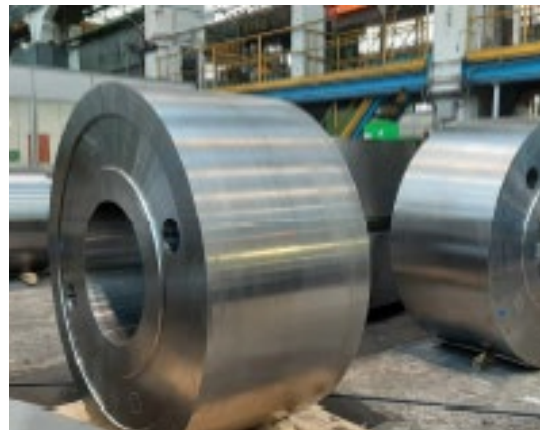
Kiln support rollers
